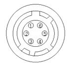
Fig. 3. 6-pin Hirose. (Seen from camera rear.)
